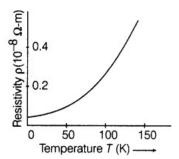
The temperature dependence of resistivity of a metal can be obtained from,  $r = r_0[1 + \alpha(T - T_0)]$
